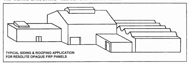
Opaque fiberglass reinforced polymer panels from Resolite are the ideal siding and roofing material for industrial and commercial buildings. Resolite premium grade polyester resin fire rated CRFS25A, Tred-Safe, RFM as well as non-fire rated CR-Acryloy, are available in a range of standard colors and profiles to meet
